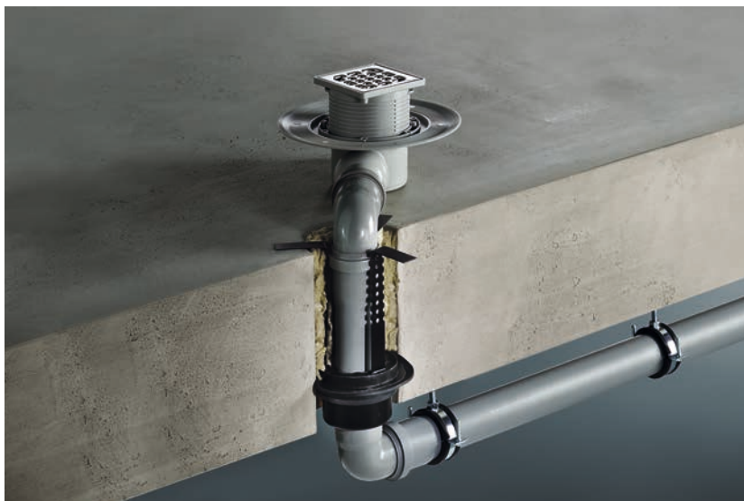
Fig. 3 – 138 Advantix pipe lead-in R 120 – mounting example
