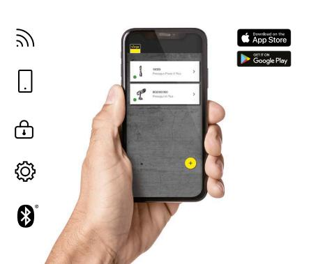
Clever: the Viega Tool Services app allows the Pressgun Picco 6 Plus to be controlled and managed interactively.
