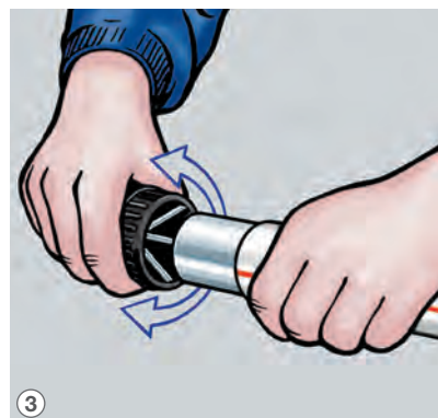
3 De-burr internally and externally. Continue with steps for Prestabo-pipe, blank (see next page)
