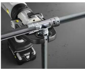
In large buildings in particular, steel pipes with threaded pipe or boiling pipe quality are the first choice when installing high-performance heating and cooling systems. Viega Megapress was developed for precisely this area of application. It connects black, galvanised, industrially painted or epoxy-resin-coated steel pipes pursuant to DIN EN 10255, DIN EN 10220/10216-1 and DIN EN 10220/10217-1 to each other – at the push of a button!
