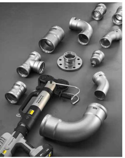
Furthermore, press connections offer a cleaner alternative as unlike threading, there is no need to use lubricating oil as part of the process. This means that the pipe and surrounding area will not require cleaning during or after installation. This also reduces the level of flushing the system will require to remove contaminants before the building is handed over.
