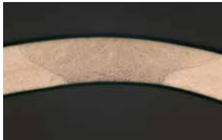
Conventional-width TIG weld seam
