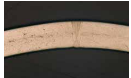
Narrow Viega laser weld seam
