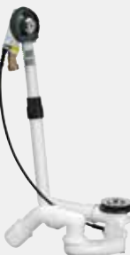
Multiplex Trio Drain/overflow functional unit flat version; only 33 mm space required behind the bathtub - for water supply through the overflow unit - plastic - without: rotatable rosette, overflow rosette, drain plug
