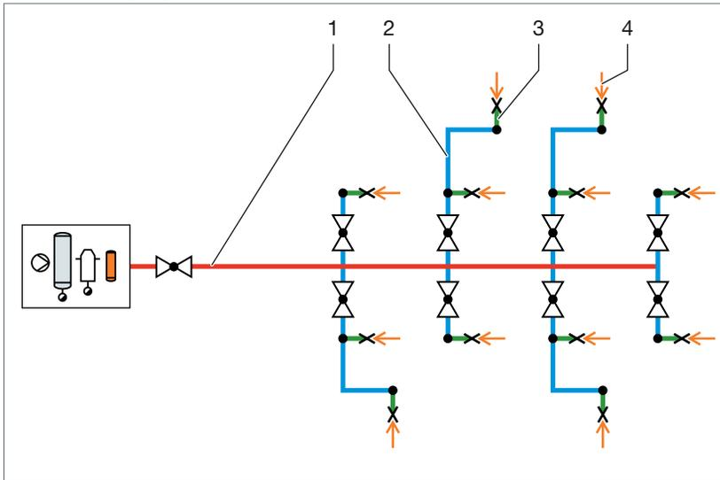
Fig. 129: Compressed air supply with single connection pipeline
