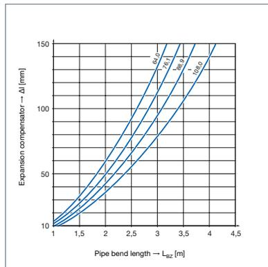
Fig. 45: Length determination for U-shaped expansion bend
