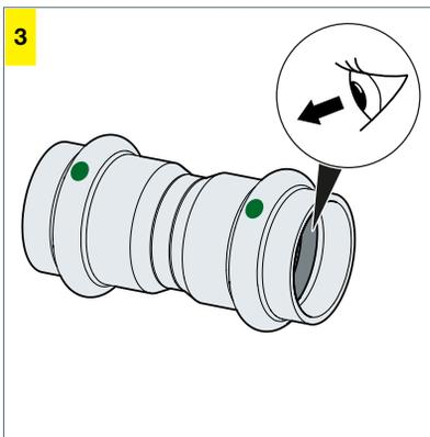
► Ensure that the sealing element is properly positioned
