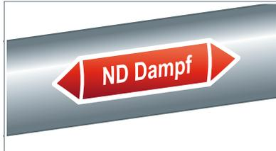
Fig. 152: Steam line with DIN 2403 marking
