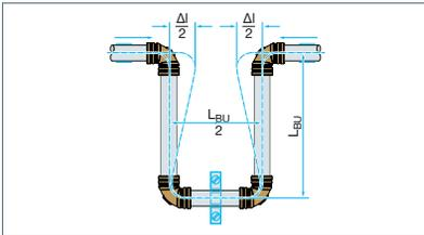
Fig. 43: U shape with expansion bend  $L_{BU}$
