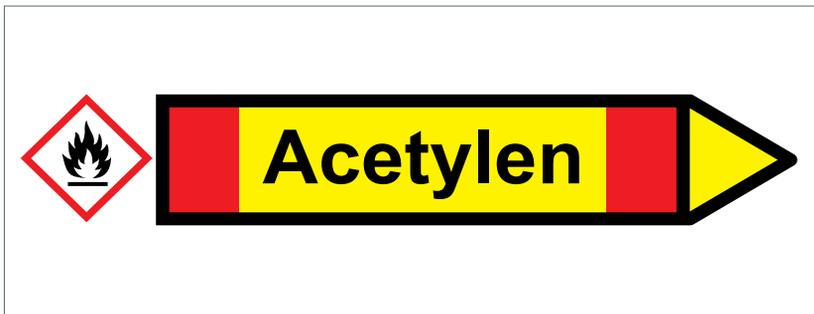
Fig. 139: Acetylene with hazard symbol
