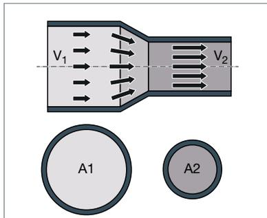
Consideration should be given to the laws of kinetic compressed air in the dimensioning of compressed air installations. The volumetric flow is calculated from the cross-sectional area of the pipeline and the flow velocity:
