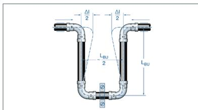
Fig. 49: U shape with expansion bend  $l_{BU}$
