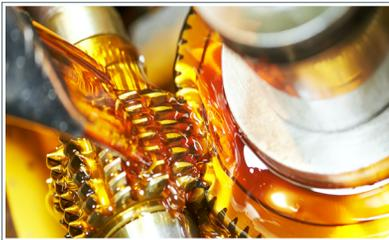
Fig. 164: Application of a cooling lubricant
