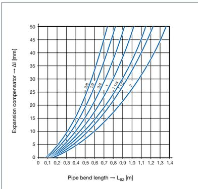
Fig. 52: U-shaped expansion bend for Megapress/Megapress S 3/8–2 inches
