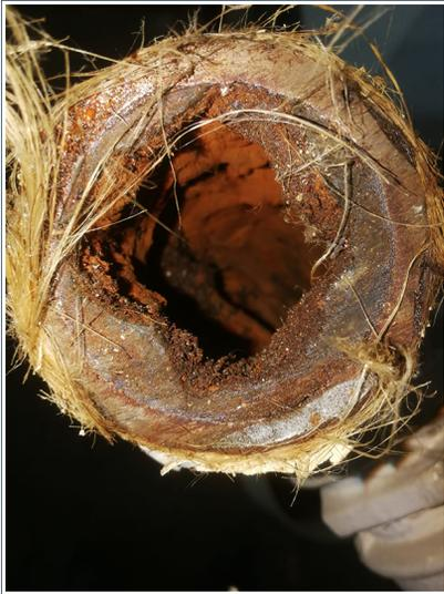
Fig. 74: Galvanised steel pipe with clearly visible corrosion
