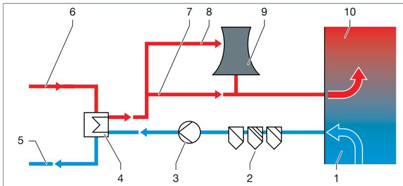
Fig. 93: Through-cooling
