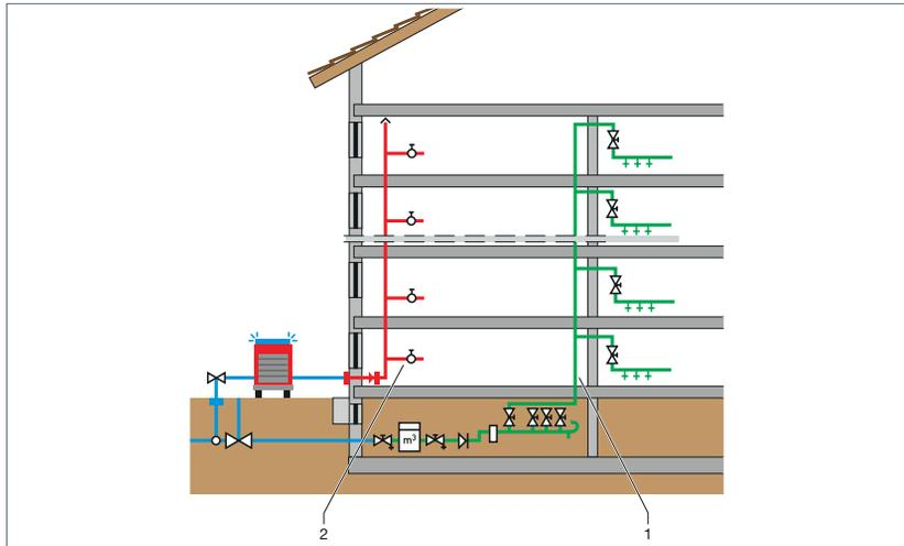
Fig. 110: Firefighting water system dry
