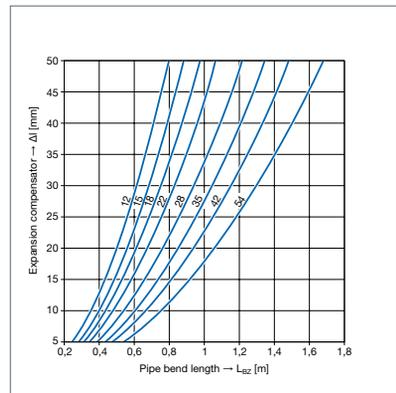
Fig. 40: Length determination for U-shaped expansion bend
