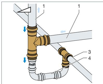
Fig. 156: Condensate loop – separation of steam and condensate
