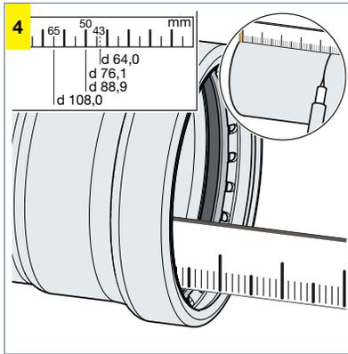
► Mark the insertion depth on the pipe.
